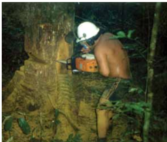
Photo 9.3. Directional felling techniques applied while felling a Greenheart ( Chlorocardium rodiei ) in RIL. (Photo P. van der Hout)
