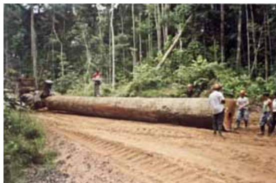
Photo 9.1. A Locust ( Hymenaea courbaril ) log of 20 m 3 proved to be too heavy to extract in one piece. (Photo P. van der Hout)
