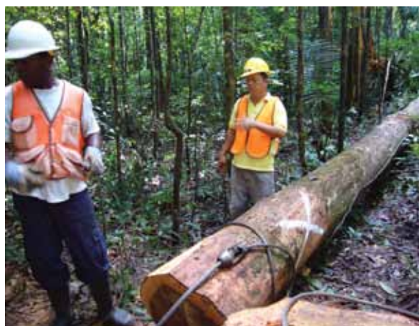
Photo 3.3. Logging technique: using choker cables for winch extraction. (Photo J. Hendrison)
