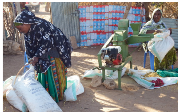
A women’s cooperative using a portable hammer mill to produce animal feed for sale, Burao, Somaliland. Women are also the main pod collectors.
