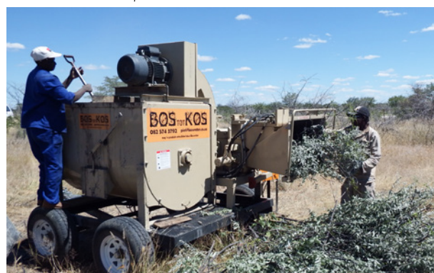
Milling and mixing invasive Combretum and Grewia species before adding feed additives, Outjo, Namibia. Specially designed mills are made in South Africa.
